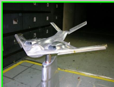
5% Scale Speed Agile Low Speed Testing NASA LaRC 14'x22' July 2009
