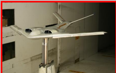
5% Scale AJACS Low Speed Testing Boeing BVWT 20'x20' Aug 2007
