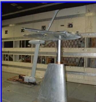
5% Scale AJACS Low Speed Testing NASA LaRC 14'x22' Apr 2008
